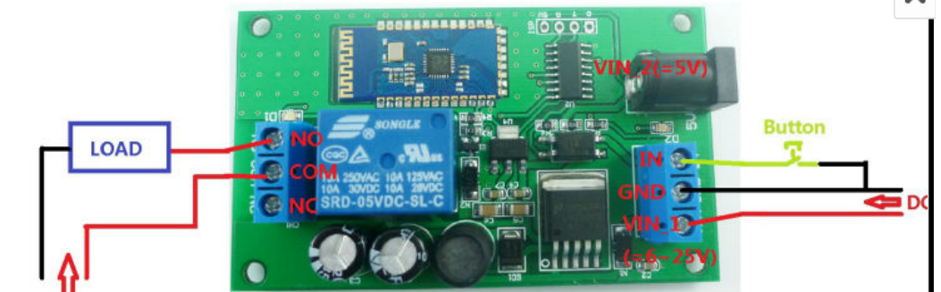
DC 1-48V OR AC 85-265V LOAD Wiring Diagram
