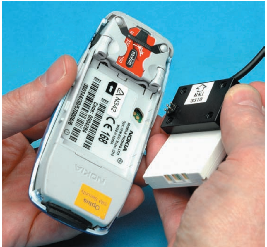
On the 3310 model, the serial interface is accessible through a hole in the rear of the case, underneath the battery. The data cable is terminated with a plastic head assembly that includes a set of spring-loaded contacts as well as tabs to retain the battery that it partly displaces.
